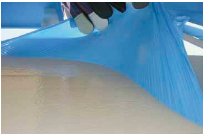
Removal of Interseal 121 from coated substrates
